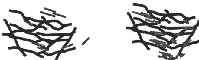
Scheme 2. A sketch of the interaction between PPQ and silica. The black thick lines symbolize the silica matrix and the gray short lines are PPQ. (a) at very low PPQ concentration, and (b) at high PPQ concentration.
