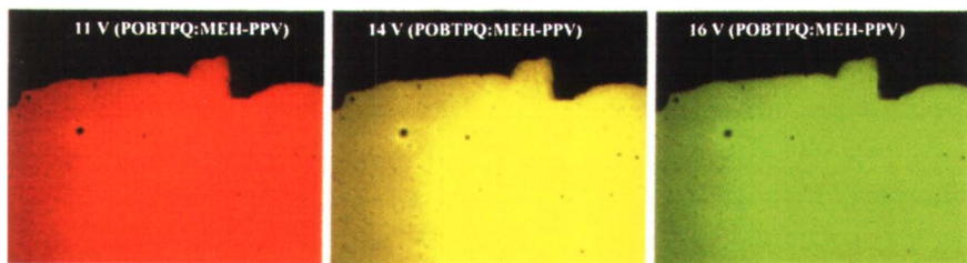
Plate 14.2. EL micrographs ( \times 10 ) of a POBTQ:MEH-PPV blend (60:40 wt%) diode at 11, 14, and 16 V.
